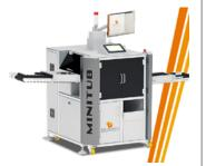
Print inspection module for Plastic tubes.
